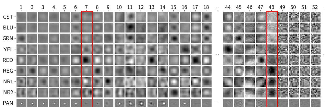
Figure 5. A subset of first-layer filter responses, column-wise re-scaled to compensate for different gains. Filters #7 and #48, highlighted, correspond roughly to vegetation and water features.
