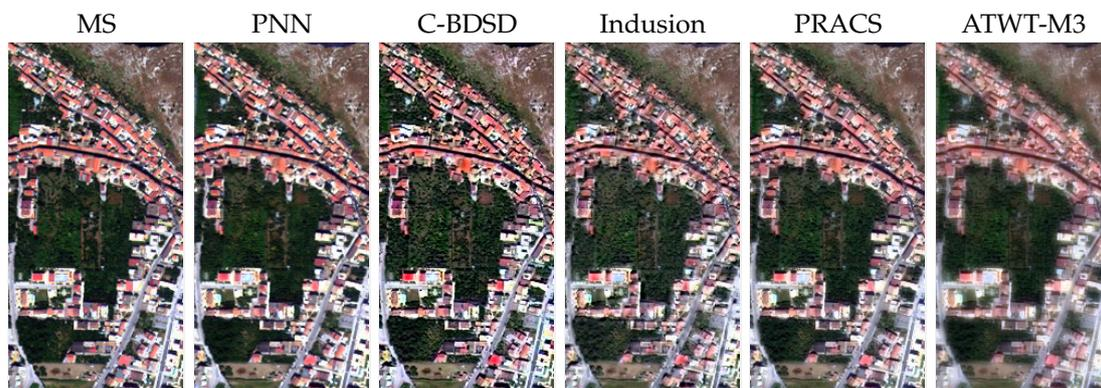
**Figure 8.** Pansharpening of a reduced resolution WorldView-2 image. From **left to right**: reference image (original MS component) output of proposed method, C-BDSB, Indusion, PRACS, ATWT-M3.
