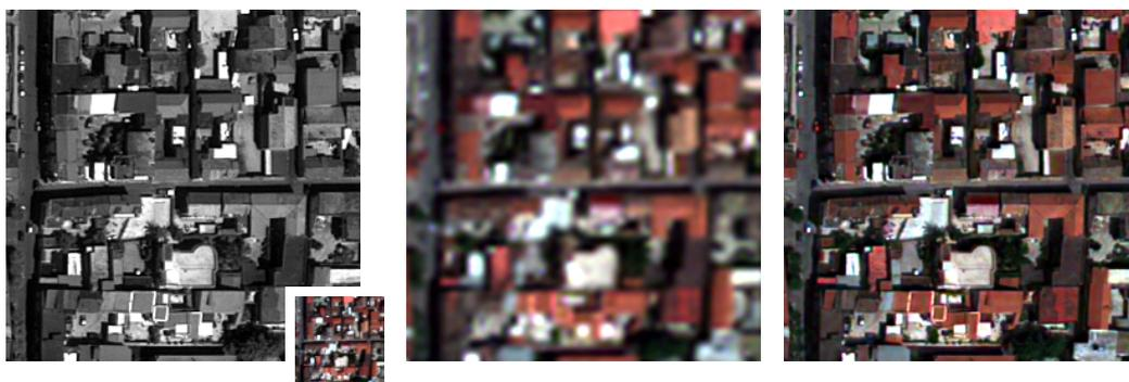
Figure 3. Sample result of proposed pansharpening method. Form left to right: input multiresolution image acquired by the GeoEye-1 sensor, interpolation of MS, pansharpened image.
