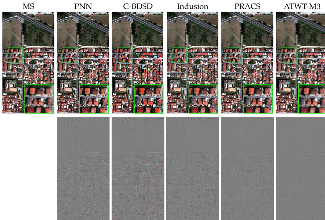
**Figure 13.** Pansharpening of a full-resolution GeoEye-1 image. **Top**, from **left to right**: interpolated MS, output of proposed method, C-BDSF, Indusion, PRACS, ATWT-M3. **Bottom**, detail images.
