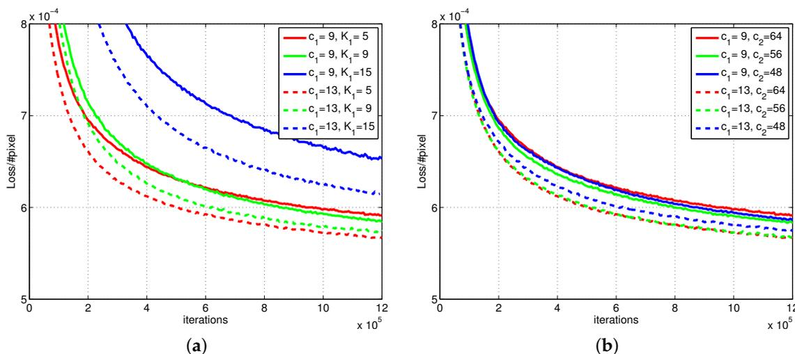
**Figure 7.** Evolution of the loss function (Equation (4)) computed on the WorldView-2 validation set during training for various architectures: (a) fixed number of filters,  $c_2 = 64$ ; (b) fixed filter support,  $K_1 = 5$ .
