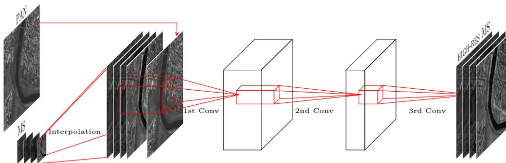
Figure 1. Basic CNN architecture for pansharpening.
