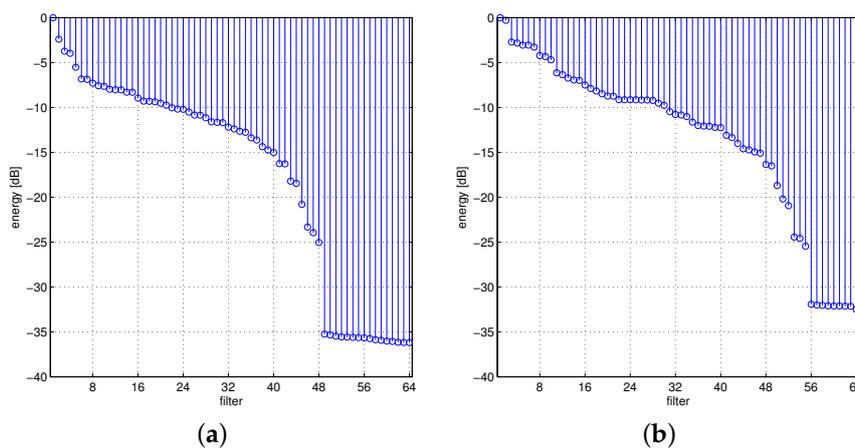
Figure 4. Energy of first-layer filters without (a) and with (b) nonlinear radiometric indices.
