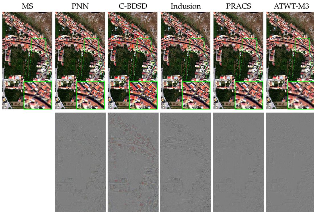
**Figure 11.** Pansharpening of a full-resolution WorldView-2 image. **Top**, from **left to right**: interpolated MS, output of proposed method, C-BDSF, Indusion, PRACS, ATWT-M3. **Bottom**, detail images.
