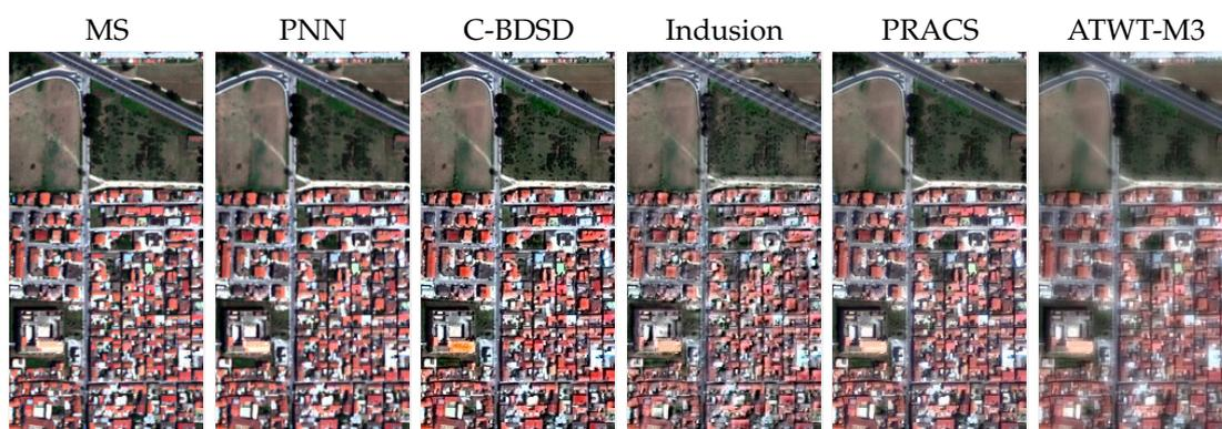
**Figure 10.** Pansharpening of a reduced resolution GeoEye-1 image. From **left to right**: reference image (original MS component) output of proposed method, C-BDSB, Indusion, PRACS, ATWT-M3.
