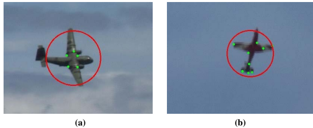
Figure 1. Sample frames showing (a) a transport aircraft and (b) an aerobatics aircraft. The green points represent detected features and the red circles show the location and scale of the tracked objects. Frames are cropped from 720 \times 576 to 400 \times 300 for brevity.
