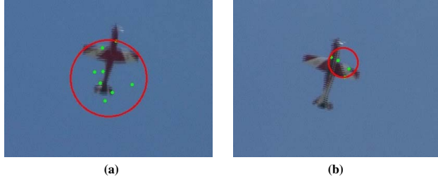
Figure 5. Two cases of error. (a) Some feature points have been extracted that do not belong to the object resulting in a shift in the location of the circle. (b) Feature points have been identified on part of the object resulting in an incorrect scale of the object. Frames are cropped from 720 \times 576 to 400 \times 300 for brevity.
