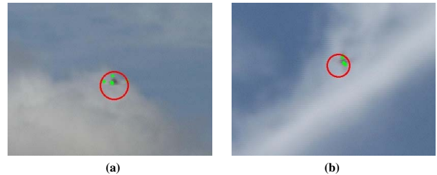
Figure 4. Two challenging cases where an aircraft, performing aerobatics, has been correctly tracked even though it was partly occluded by clouds. Frames are cropped from 720 \times 576 to 400 \times 300 for brevity.
