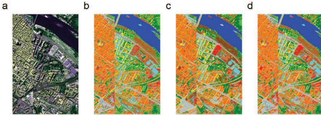
**Fig. 6.** (a) False color original image of Pavia center. (b) Classification map using the RBF kernel. (c) Classification map using the EMP. (d) Classification map using the proposed kernel where  $\lambda = 20$ .
